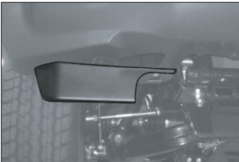
Figure 6. Reattach Bumper Lower and Plastic Shields
